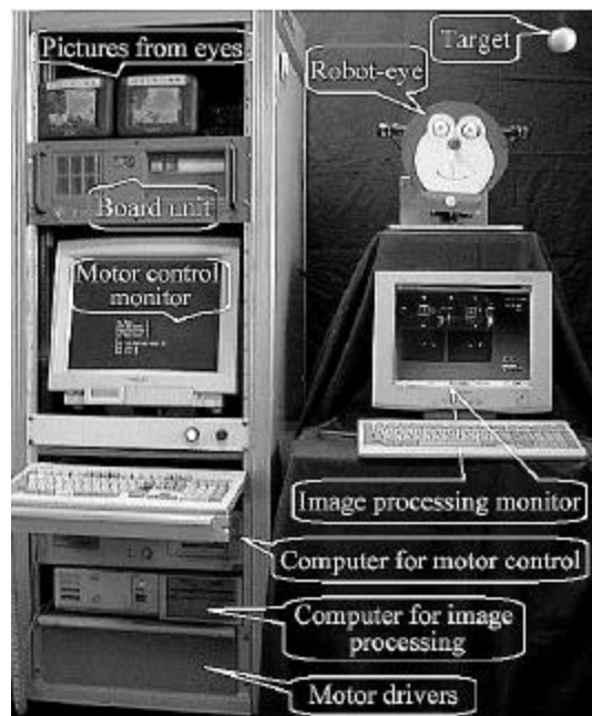
Fig. 11 Entire exterior of robot-eyes system
